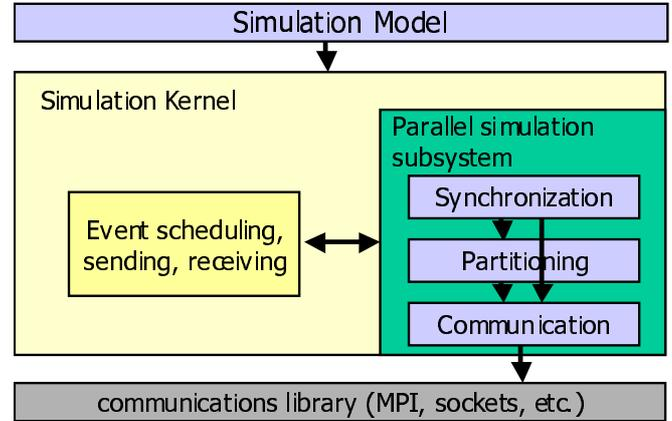
Figure 6: Architecture of OMNeT++ PDES implementation
