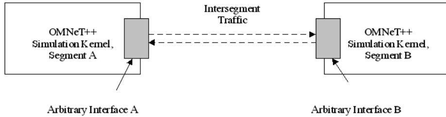
Figure 2: Sending/receiving functions are invoked by the simulation kernel, and handled by an arbitrary parallel interface.
